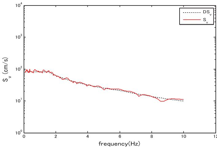
FIGURE 9  $S_v$  and  $DS_v$  of the ground motion.
