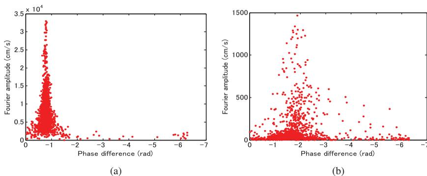
**FIGURE 1** Phase differences as a function of the Fourier amplitude for records at a) the Hino site (epicentral distance = 7 km) and b) the Taishi site (epicentral distance = 227 km) from the Tottoriken seibu earthquake (data for 0.1–10.0 Hz are used).
